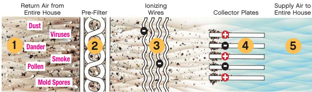
The Electronic Air Filtration System is Carrier's most efficient, removing up to as much as 68% of the dust and pollutants from your indoor air.
